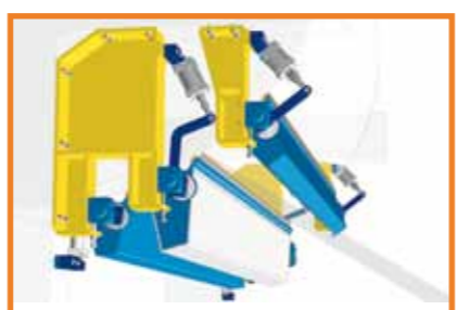
4 Cutting, Creping and Cleaning Doctor in Yankee
