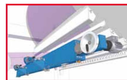
19 LANCUT Automatic dry Tail Cutter with rotating saw
